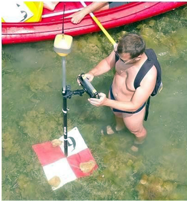
Fig. 4. – Target positioning with Topcon HiPer HR.
