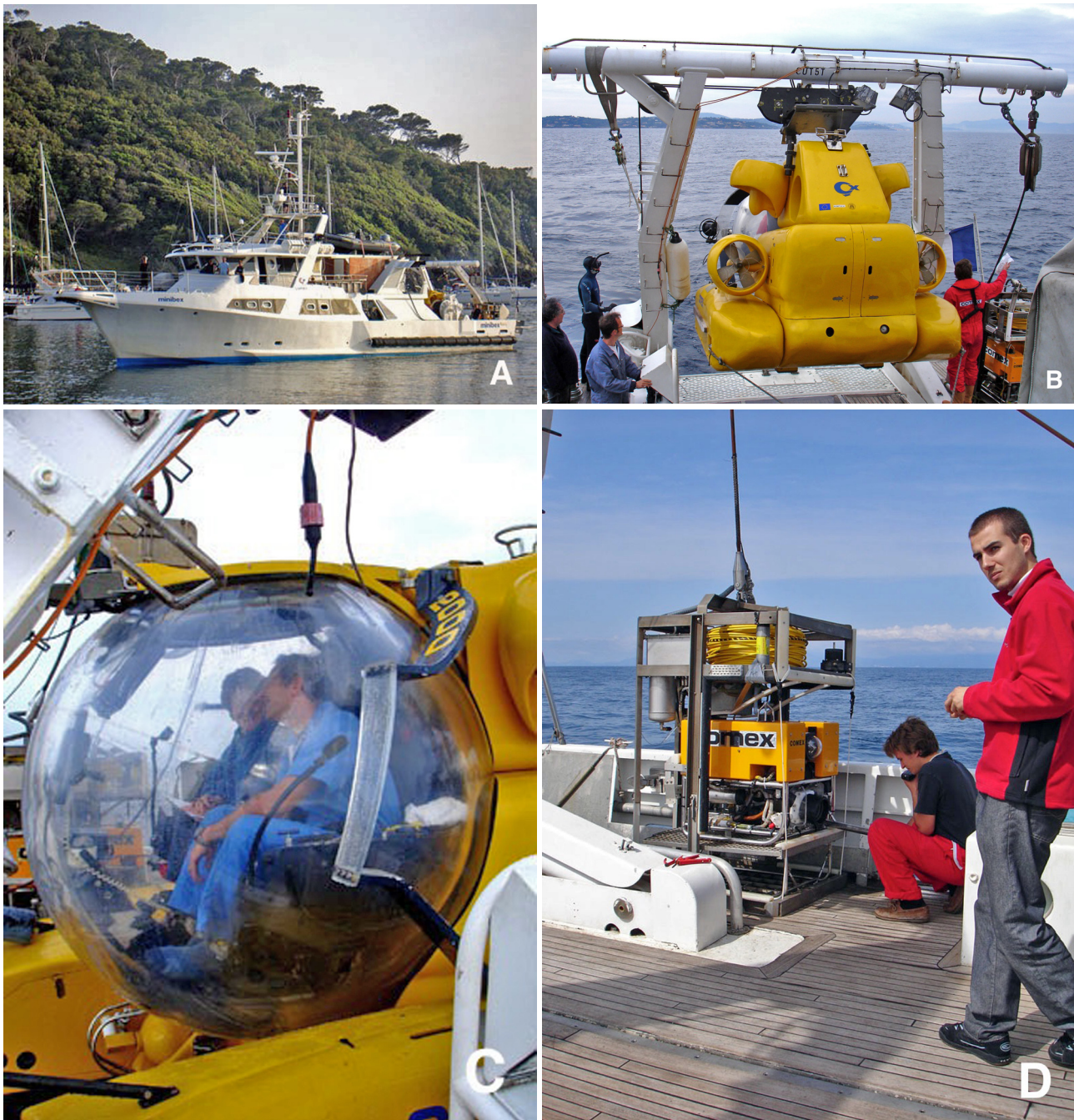
Fig. 1. – A: Oceanographic ship “MINIBEX” (COMEX); B and C: Submersible “REMORA”; D: ROV “ACHILLE”.
